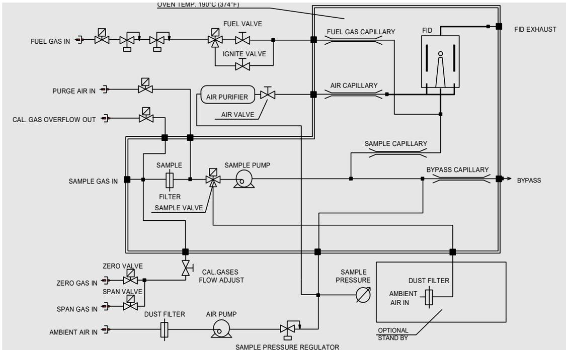
Complete Flow Diagram shown with Back Purge Sample Filter
