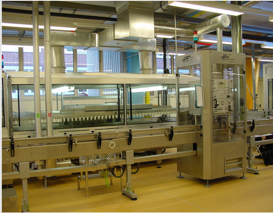
250 CPM Leak Tester shown installed after a hot water bath
