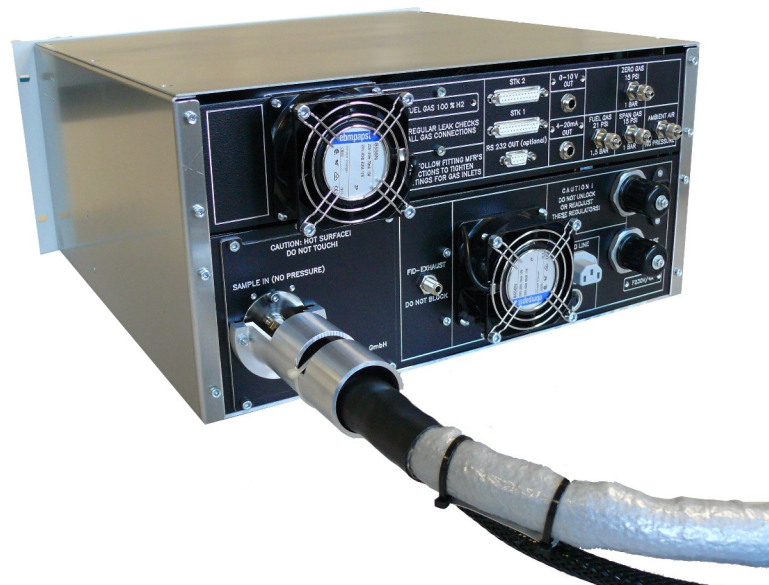
Rear Panel Shown with 1.5 mm Inside Diameter Heated Sample Line for Shortest Response Time
